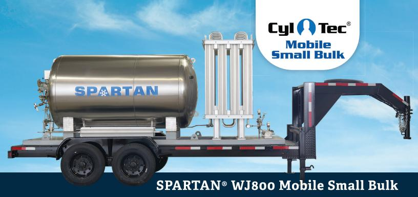
Transport up to 720 gallons of liquid product directly to your job sites. CGA 341 road relief circuit allows safe transport of Nitrogen, Oxygen, and Argon.
