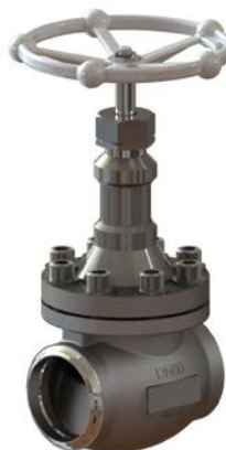
DN80 Stainless Steel Globe Valve Extended Stem with Butt Weld Ends
